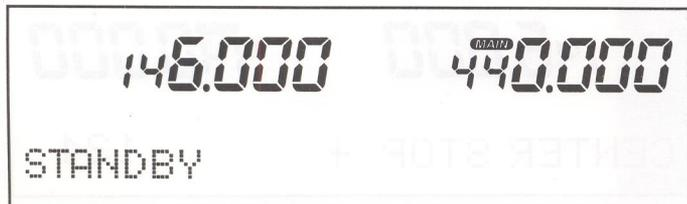
In the alignment routine, each adjustment is selected in sequence by moving the joystick *right* or *left*. After this point, alignment is performed by injecting a signal of a required frequency or level and transmitter output power level adjustments are performed moving the joystick *up* or *down*. When the proper input or output level has been reached, the setting is saved by pressing *inward* on the joystick or else the **HOME** button.
