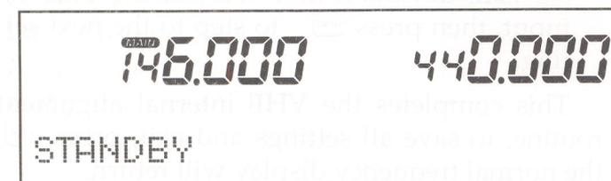
The alignment routine is active, and the display appears as below, awaiting joystick input.
