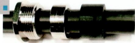
Slip the nut, the pressure ring and the rubber gasket over the cable end.
