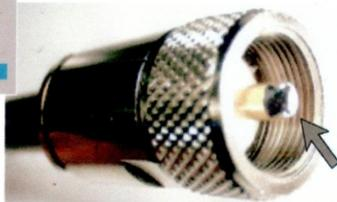
Solder the center conductor carefully to the connector tip.
