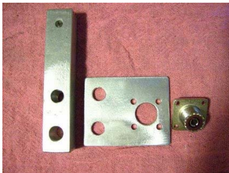
Plate bracketed by the base block and SO-239 connector.
