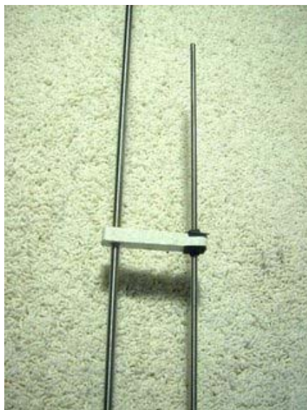
Speed nuts trapping the spacer.
