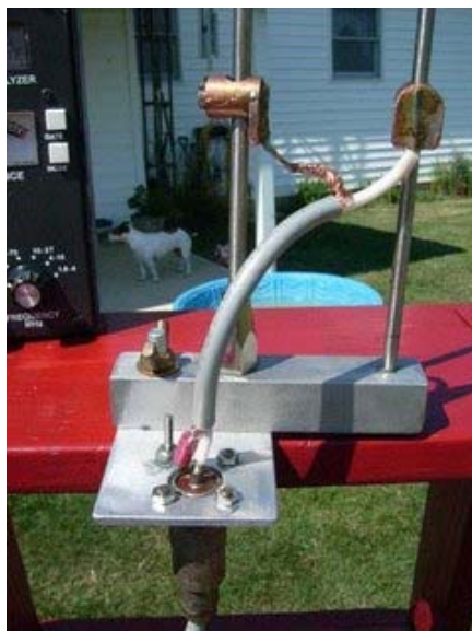
Rear view of coax taps & SO-239 connections
