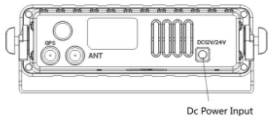
④ Insert GPS antenna / external main antenna.
