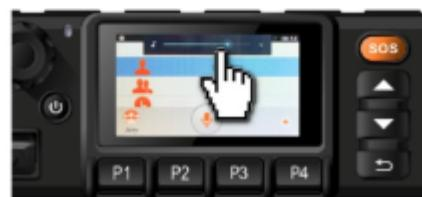
**4. It will alarm automatically after 2 seconds when emergency and pressing SOS button.**
