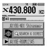
While [X] is flashing, briefly press the 💽 key to re-establish connection to the local node. When any local node cannot be found, [X] will disappear in 30 seconds.
