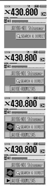
When ► is displayed, rotate the DIAL. Call signs of nodes and rooms on the Internet you previously connected to flash.
