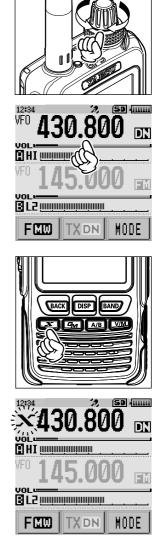
When a local node is found, [X] is lit solid, and the node name and city name appear on the bottom part of the screen.
