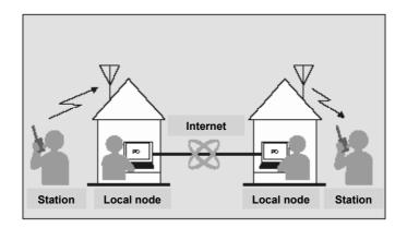
In addition to the WIRES features, WIRES-X also supports digital communications. Using WIRES-X, you can transmit and receive digitalized data such as text, image data and audio.
