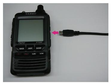
6. While pressing down AB, connect the AC adaptor connector to the FT2DR/DE EXT DC IN terminal.
