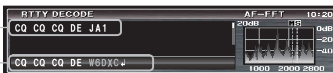
AF-FFT display (see page 40) (“Spectrum” or “Waterfall” display)
