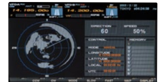
■ Antenna Bearing Indication using Great Circle Map
