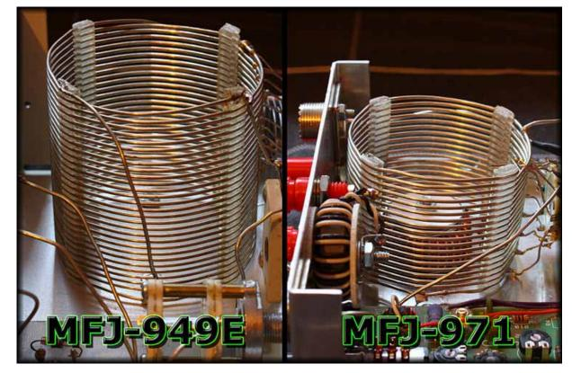
The MFJ-949E inductor has 27 turns, 75mm long and 75mm diameter which is about 37µH. The MFJ-971 inductor has 17 turns, 43mm long and 66mm diameter which is about 17µH. Adding on the extra inductance means we have a max inductance of around 27µH which allows matching on 1.8MHz. Air inductance coils can be calculated <u>here</u> and the T130-2 toroid <u>here</u>.
