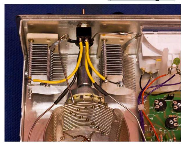
Usually, the signal comes off the PCB and straight into the 'transmitter' capacitor and the output of the 'antenna' capacitor goes to the coax/wire connection on the rear. The switch has been added to provide a way to bypass the tuner section. A drawing of the DPDT switch wiring is below.
