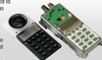
**PERFORMANCE** A premium radio design like the TK-480/481 portables use state-of-the-art surface mount technology, multiple layer epoxy PC boards, high-level integrated circuits and hybrid components to create a symphony of compact, rugged and power efficient performance.
