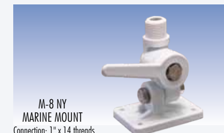
M-8 NY MARINE MOUNT Connection: 1" x 14 threads Dimension L x W x H: 67 x 94 x 124 mm Weight (approx.): 330 gr Material: Nylon, Stainless steel hardware M-8 NY marine mount ..... P/N 2503301.00
