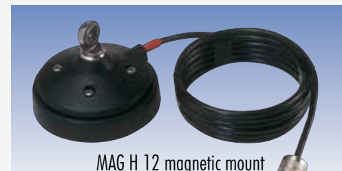
MAG H 12 magnetic mount Frequency Range: from DC to 500 MHz Overall Size: Ø 92 mm Materials: Ferrite magnet, Chromed Brass, Nylon, Rubber protection Cable / Connector: 3.6 m RG 58 / PL 259 R male MAG H 12 S ..... P/N 2502502.01 MAG H 12 S Black ..... P/N 2502502.02 MAG H 12 3/8 ..... P/N 2502502.03 MAG H 12 PL ..... P/N 2502502.05
