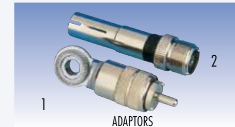
ADAPTORS 1. DV - PL adaptor: from PL-259 mount to DV joint whip ..... P/N 2506806.00 2. Rx adaptor: from portable transceiver to SO-239 for cable output ..... P/N 2506906.00
