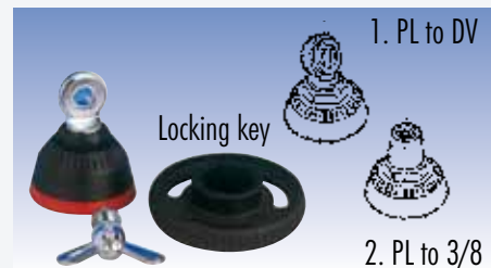
Locking key Type: Magnetic mount adaptor Material: Chromed zamac, Nylon Connection: 1. PL-259-male to DV joint (Black available) 2. PL-259-male to 3/8" thread 1. MAG-DV adaptor ..... P/N 2504502.01 1. MAG-DV adaptor black ..... P/N 2504502.02 2. MAG-3/8 adaptor ..... P/N 2504502.03
