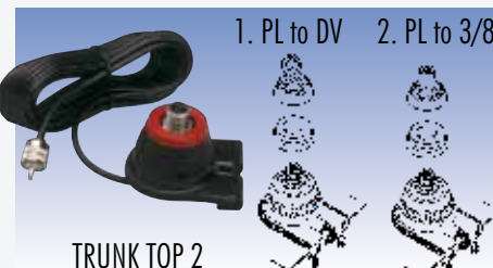
TRUNK TOP 2 Type: Trunk mount Cable / Connector: 5.5 m RG 58 / UHF-male Connection: UHF-female, 3/8" Thread or DV joint 1. PL or DV chrome ..... P/N 2504406.12 1. PL or DV black ..... P/N 2504407.13 2. PL or 3/8 Chrome ..... P/N 2504406.14 2. PL or 3/8 Black ..... P/N 2504407.14
