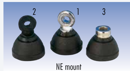
NE mount Overall Size: Ø 36 mm Mounting Hole: Ø 12.5 mm Materials: Chromed Brass, Nylon, Rubber 1. NE Chrome ..... P/N 2500202.01 2. NE Black ..... P/N 2500202.02 3. NE 3/8 ..... P/N 2500202.03
