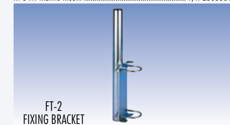
FT-2 FIXING BRACKET Top size: Ø 38 mm for antenna fitting Bottom Size: Ø 42/50 mm for fitting on the mast Weight (approx.): 1100 gr Material: Galvanized steel FT-2 Universal ..... P/N 2510004.00
