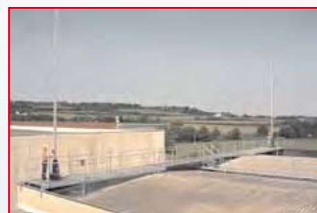
Open site antenna measurement
