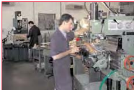
Moulds and equipments production: milling machine and spark erosion machine
