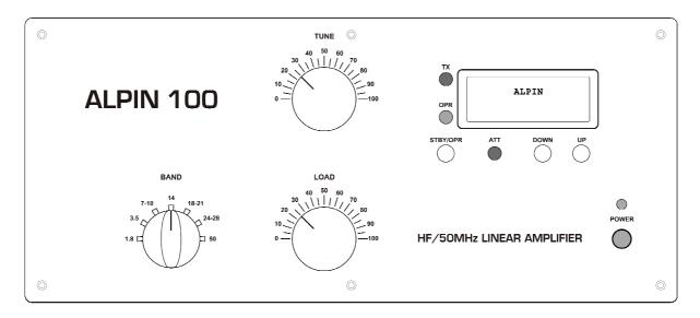
The front panel is divided into two parts: One for tuning and band switching (left) and another for the visualization.(right)
