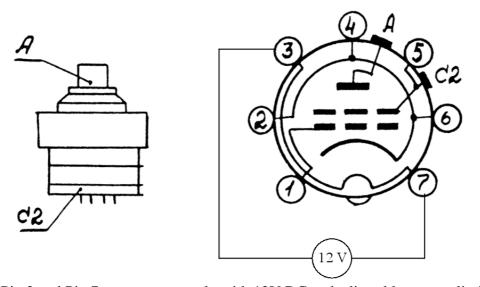
Connect Pin 3 and Pin 7 to a power supply with 12V DC and adjustable current limiter. Supply each of the following currents for 3 minutes: 0.5 A / 1 A / 2 A / 3 A / max current ca. 4 A.
