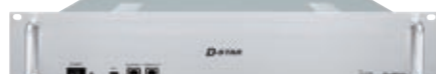
ID-RP2V: Modulo RF a 1.2 GHz - DV ID-RP2000V: Modulo RF a 144 MHz - DV ID-RP4000V: Modulo RF a 430 MHz - DV
