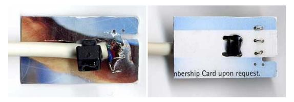
This plug was made out of an old plastic. Just cut it into the necessary form and drill six holes for the cable ends. Another two slits are used for a pull relief for the cable. The ends are fixed by superglue or two-component glue. Be careful not to produce a short circuit by accidently connecting the ends of the data cable.
