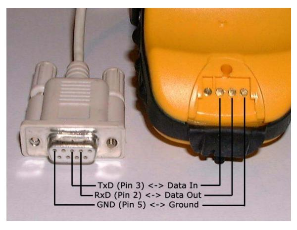
On that picture you can see how simple the data cable is build. Only 3 connections of the serial cable are to be connected directly to the eTrex. Fortunately Garmin forewent to use a proprietary hardware solution (beside that awkward plug).
