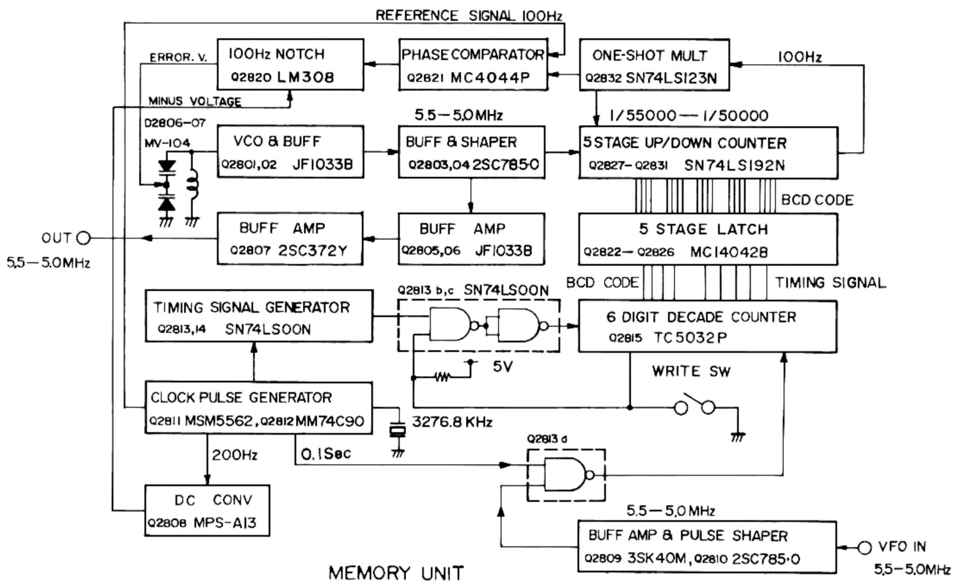
is amplified by Q<sub>2805</sub> and Q<sub>2806</sub> (both **JF-1033B**) and Q<sub>2807</sub> (**2SC372Y**), and fed through a diode switch to the PLL UNIT (replacing the VFO signal).
