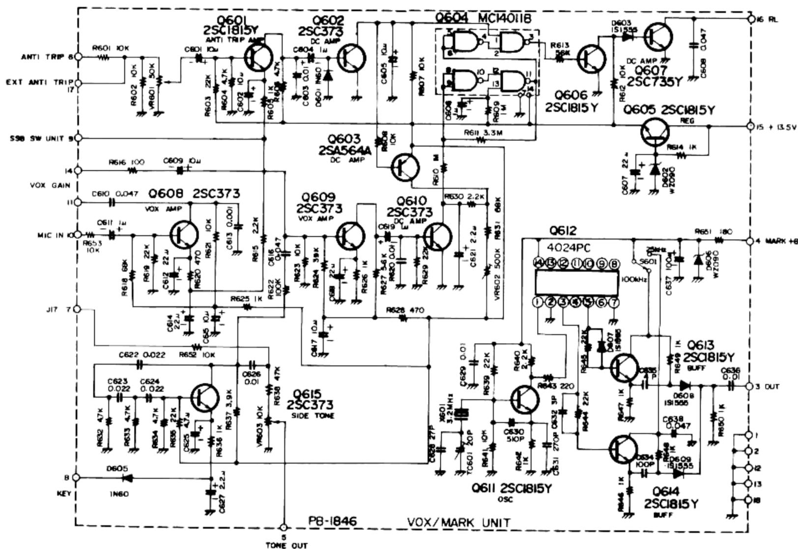
The VOX GAIN control  $VR_1$  on the front panel provides adjustment for relay sensitivity, and  $VR_{601}$  controls antitrip sensitivity. Relay hold time is determined by delay control  $VR_{602}$ .
