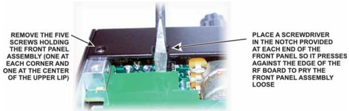
Figure 63. Removing the Front Panel.
