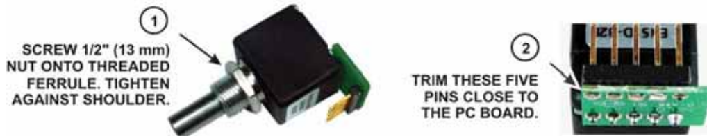
Figure 43. VFO B Encoder Assembly Preparation for Installation.
