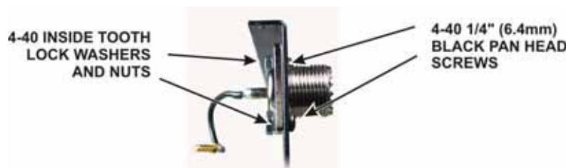
Figure 18. Mounting the ANT1 Connector.
