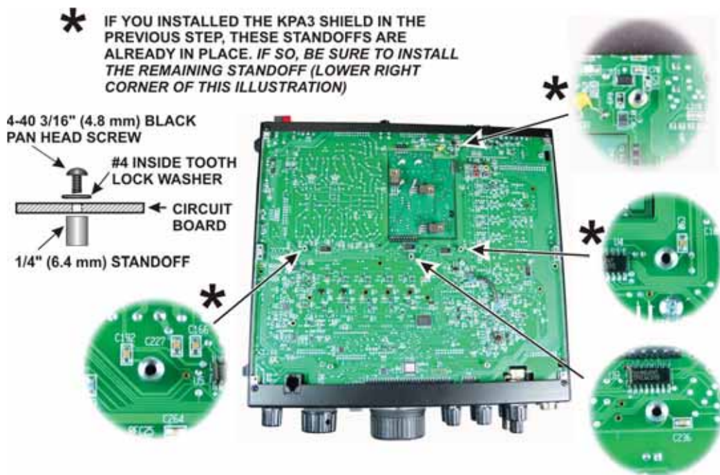
Figure 81. Installing Standoffs on RF Board.
