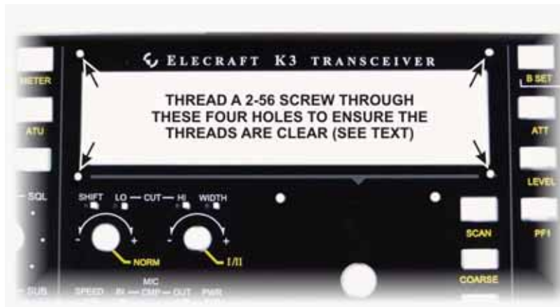
Figure 39. Checking 2-56 Threaded Screw Holes.
