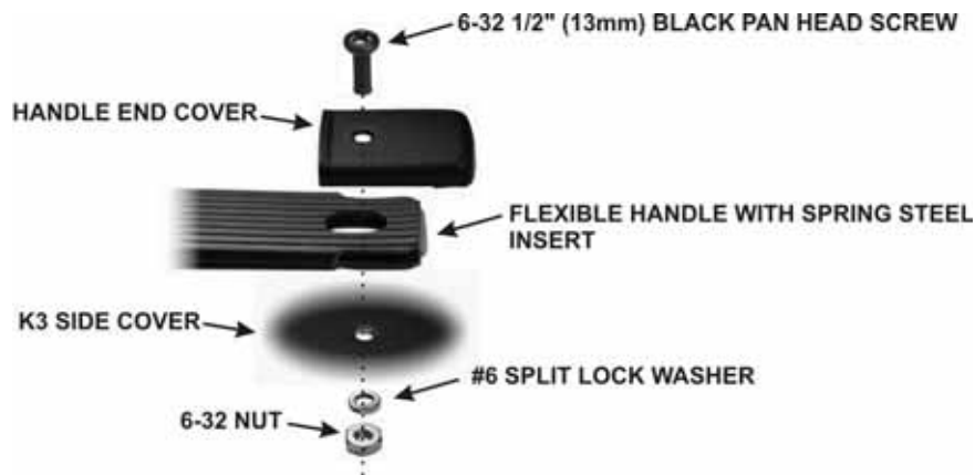
Figure 15. Installing Side Handle Mounting Hardware.
