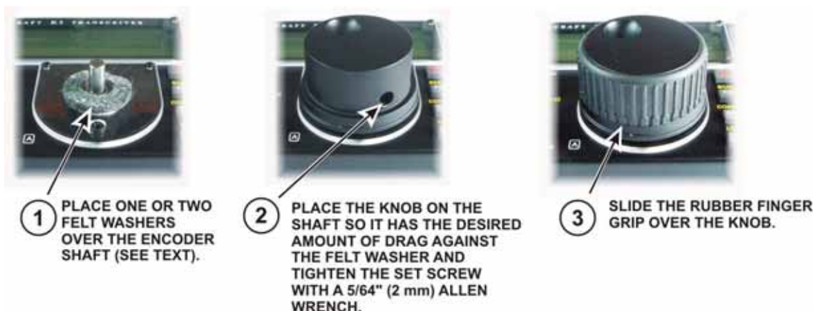
Figure 49. Mounting the VFO A Tuning Knob.
