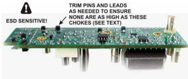
Figure 69. Checking Lead Lengths on KREF3 Board.
