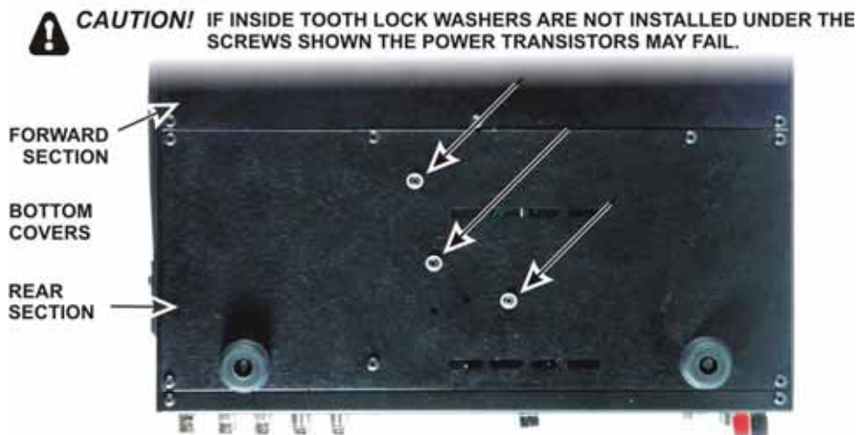
Figure 90. Checking Power Transistor Mounting Hardware.
