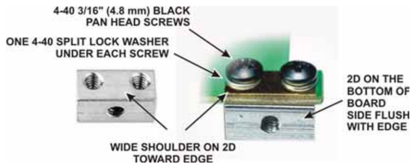
Figure 6. Installing 2D Fasteners on RF Board.
