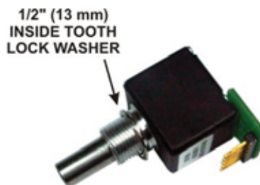
Figure 41. VFO A Encoder Assembly Preparation for Installation.
