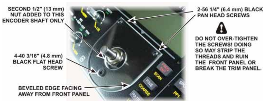
Figure 44. Mounting VFO A Trim Panel.
