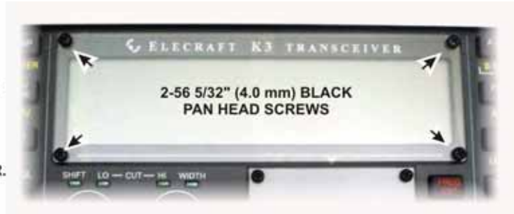
Figure 46. Installing LCD Cover.
