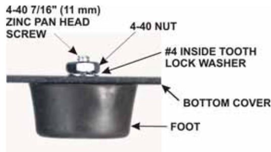
Figure 83. Installing Rear Feet.
