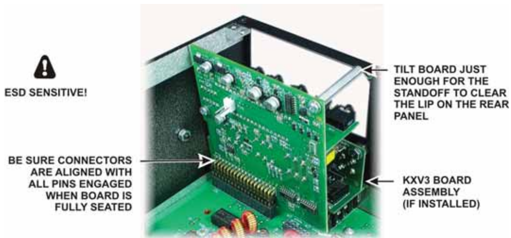
Figure 33. Installing KIO3 Main Board.
