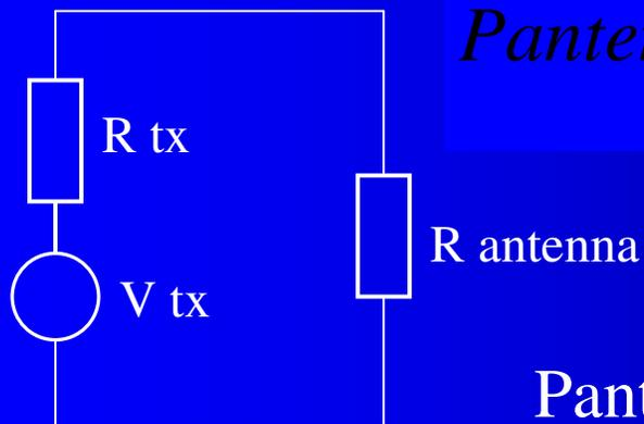
$$P_{antenna} = R \cdot I^2 = V^2 \cdot \frac{R_{antenna}}{(R_{antenna} + R_{tx})^2}$$
