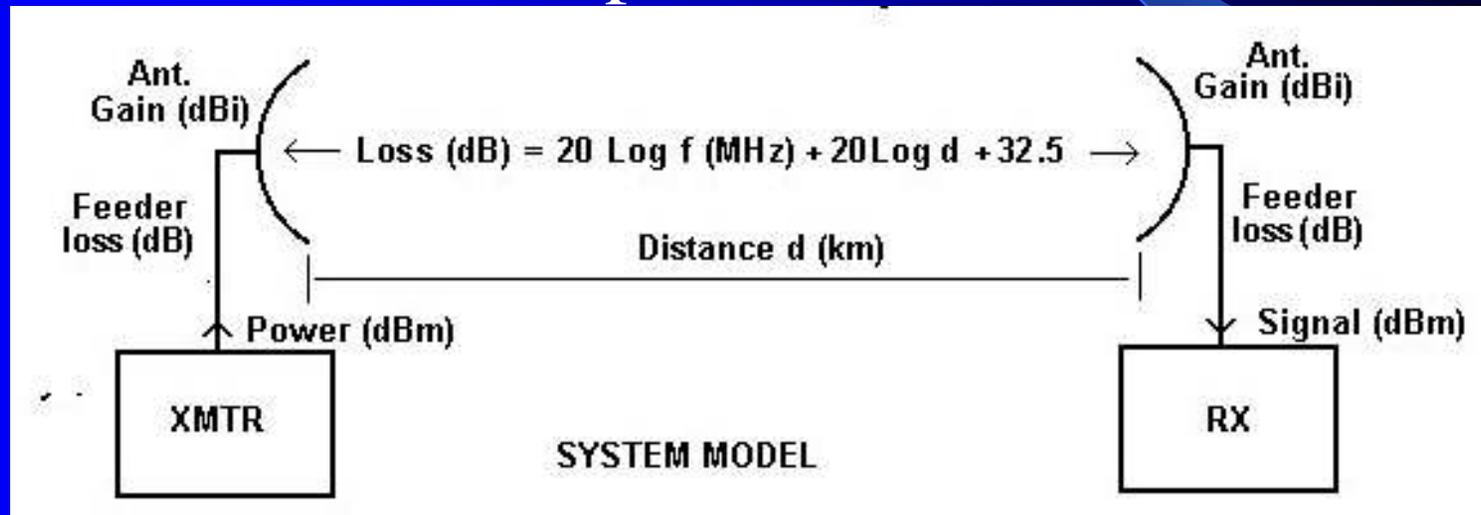
$$P_{tx} - \text{FeederTxLoss} + \text{AntTxGain} - \text{PathLoss} + \text{AntRxGain} - \text{FeederRxLoss} = P_{rx}$$
