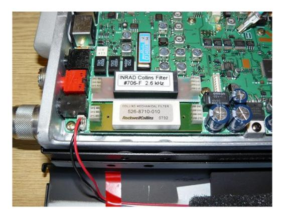
For selecting the 3.8 kHz filter in RX, quickly touch the FUNC button and turn the SELECT knob to MENU MFn where you can select CFIL (2.3kHz ceramic filter) or the 500 (now 3.8 kHz Collins filter). This gives you a very open and rich sound in SSB.
