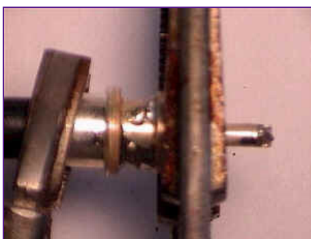
Soldered Center Conductor and Top Two Holes
