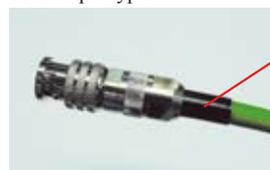
Confirm the condition from the connector shrinkable tube abt. 15mm remained
