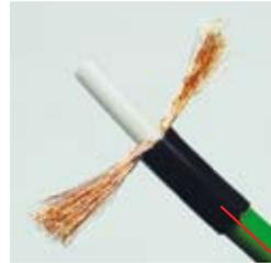
Adjust by covering with shrinkable tube as photo shows, in case of O.D. thin type cable like multi type cable, etc.
