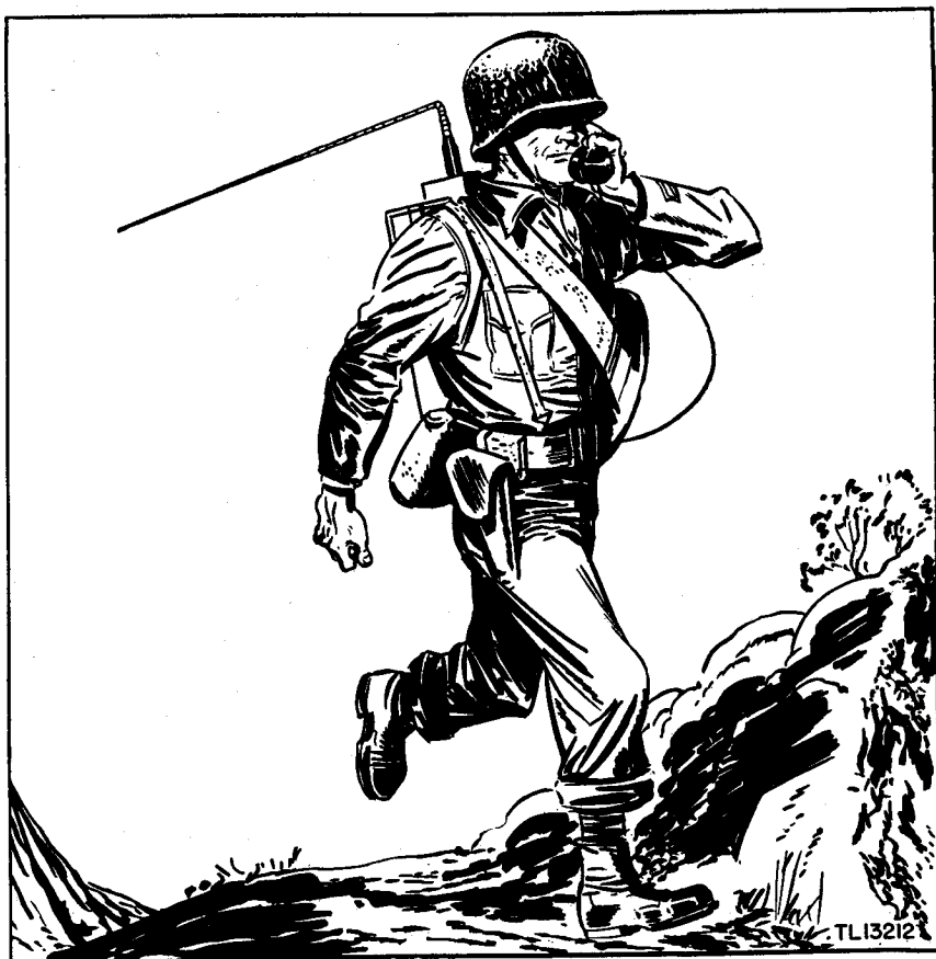
Figure 27. Do not operate with the antenna horizontal; keep it vertical.
