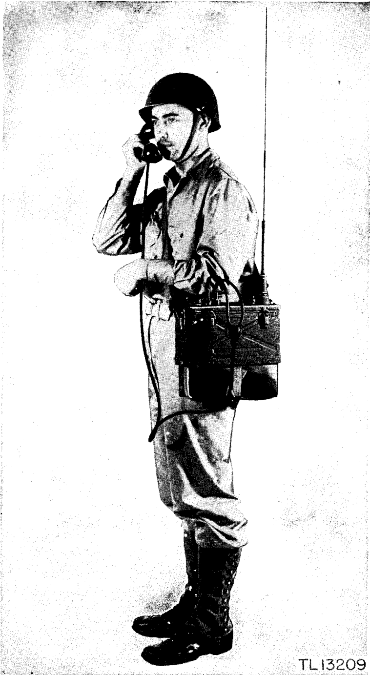
Figure 19. Radio Set SCR-300-A, lightweight installation.
