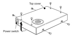
③ After installing the optional unit or any internal setting is finished, replace the top cover, cables and screws to the original position.
