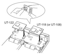
3 Replace the top cover, cables and screws to the original position.
