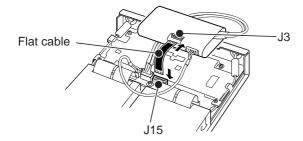
⑥ Remove the protective paper from the supplied velcro<sup>®</sup>, then attach it to the UT-106 and the shield case of MAIN board.
