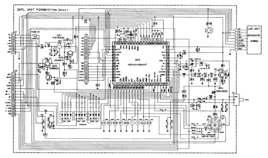
RESISTOR VALUES ARE IN n. 1/10W: CAPAVITOR VALUES ARE IN NF. 500V: UNLESS OTHERNISE NOTED. (THEAPACITORS ARE TANTALUM.
