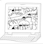
This transceiver includes a TNC and a program for dealing with data formats supported by the APRS. That is, you need no other equipment to transmit, receive, or display APRS packets. You do not need even a GPS receiver if you enter position data manually to transmit. For hams who want to fully enjoy APRS operations, this transceiver has connection ports with a personal computer and a GPS receiver. This manual, however, does not describe APRS operations which require a personal computer.
