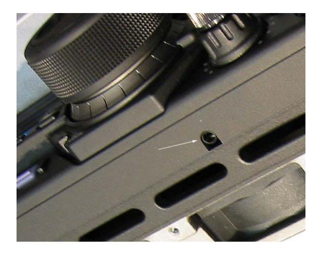
Your FT-Meter requires 12 volts DC at 100 ma to operate the light. Connect a suitable power supply to the 2.5 x 5.5 mm coaxial DC input jack using the provided 2.5 x 5.5 mm jack coaxial power connector (center positive). If you don't want to use the meter light, simply leave the power jack unconnected; the meter itself is a passive device and will work fine without the 12 volt input.
