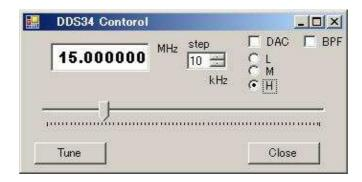
You can tune with 3 way. inputting frequency to form window, and click Tune button.
