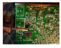
painting flux enough and touch slightly with solder iron and dissolve solder. Please let iron ahead slide on a pin slowly. When solder melts, Comming to follow an iron by surface tension. sliding solder iron few times enough.
