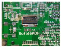
tweezers from the gap of the tape, and please match a land with a pin precisely. I perform position laying upon till I understand while confirming it with a loupe.
