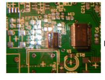
Let AD9834 fix with tape. Soldering the both ends of the pin.
