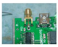
SMA Jack confirms whether the back and a list become straight and solders it from a core line. Please carry away solder after the pad of the bottom heated enough.
