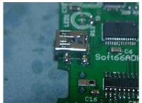
Soldering other pads completely.
