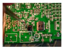
Chip part becomes parallel. In the state that declined, Causing the poor solder. Painting the whole board with a flux. Soldering other side of chip parts.
