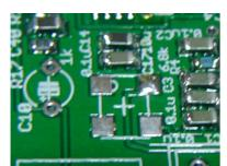
Please confirm the installation course of the oscillator by surface notation. At first, for installation, Piling solder in one place of the pad. Painting the back of OSC with a flux. The reason is because solder makes it easy to seep.
