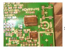
Soldering one place of other side. Dissolving solder from this side.
