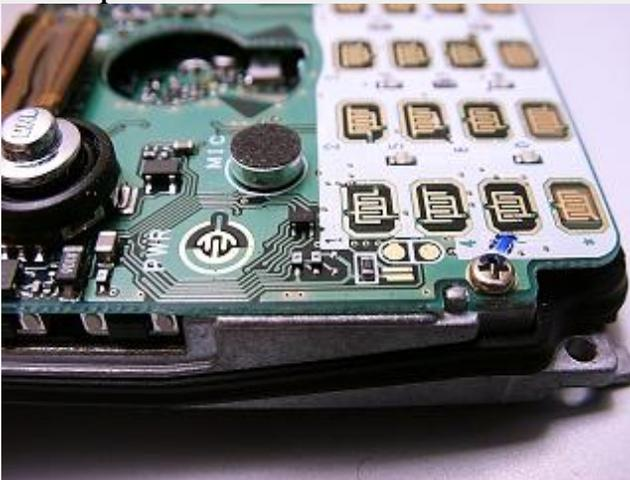
9. Remove only the top diode. There still should be a diode in the middle position and the bottom position should be left empty as original.
