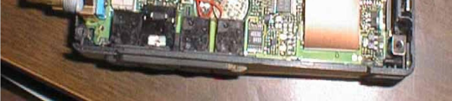
8. Pull the brown part of the ribbon cable connector upwards using your fingernail or small screwdriver. This will release the ribbon cable.
