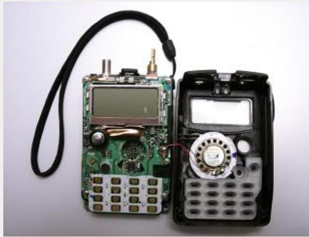
8. With the radio opened up like a book, look at the left hand side of the PCB just to the left of the PCB mounted microphone. You should see two diodes and also a open pad just below were another diode could be fitted.
