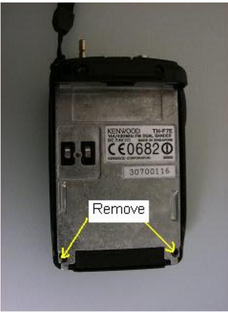
7. To open your radio's case. It's best to gently open the radio from the bottom until you have a gap of about 10mm. Then hold the front panel in the palm of your left hand and gently slide the main body of the radio downwards with your right hand, until the aerial and frequency change encoder shaft are clear of the holes in the top panel of the radio. Take care not to open the radio too fast, because the internal speaker wires are very short.
