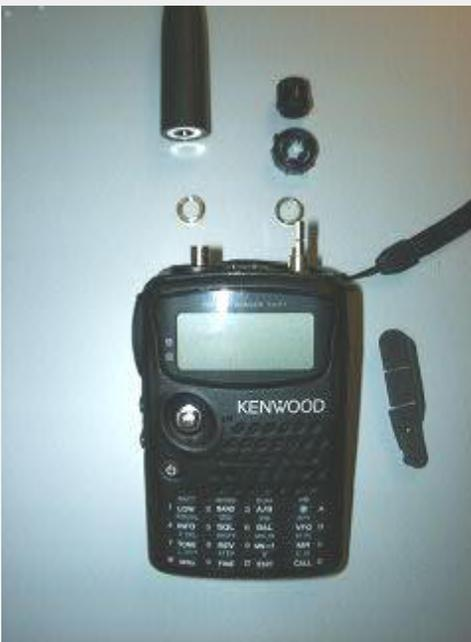
6. With the battery removed, look at the rear of the radio and remove the two screws at the bottom.
