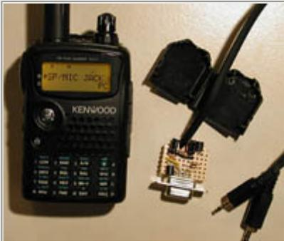
Torbjörn Söderberg (SM4XDJ) in Sweden managed to fit the entire circuit board inside a DB-9 Clamshell-style connector for his TH-F7E (European version of the TH-F6A). More photos [here](#).
