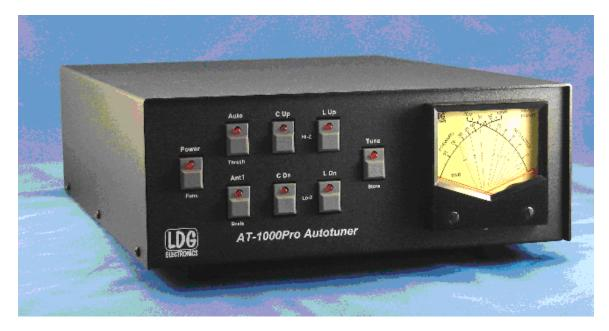
The Power switch does not turn the tuner completely off. It places it in a low-current "sleep" mode. In the Off mode (Power LED is off), the tuner is in bypass, routing RF directly from your amplifier to the antenna with no matching. On power-up, the tuner automatically restores the last tuned setting.
