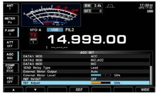
A very accurate frequency counter is required to calibrate the frequency of the transceiver. However, a rough check may be performed by receiving radio station WWV, WWVH, or other standard frequency signals.
