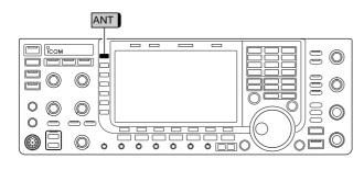
The IC-7700 has 4 antenna connectors for the HF/50 MHz bands, [ANT1], [ANT2], [ANT3], and [ANT4].
