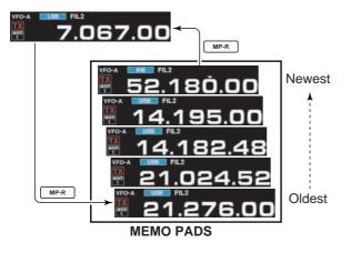
You can store the readout frequency and operating mode by pushing  $\fbox{MP-W}$  .
