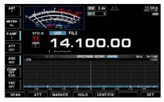
Displays signals within the specified frequency range. The selected frequency band conditions can be observed at a glance when using this mode.
