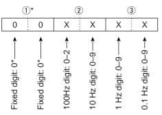
\*Not necessary when setting a frequency.
