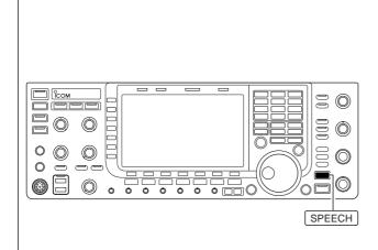
The IC-7700 has built-in voice synthesizer to announce the frequency, mode, etc. (S-meter level can also be announced—p. 12-15) in clear, electronically-generated voice, in English (or Japanese).
