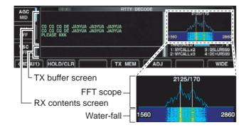
A DSP-based high-quality Baudot RTTY encoder/decoder is built-in to the IC-7700. When connecting a PC keyboard (p. 2-6), RTTY operation can be performed without an external RTTY terminal, TNC or PC.
