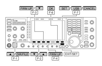
When updating the firmware with the USB-Memory, no IP address or subnet mask settings are necessary.
