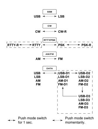
SSB (USB/LSB), SSB data (USB data/LSB data), CW, CW reverse (CW-R), RTTY, RTTY reverse (RTTY-R), PSK, PSK reverse (PSK-R), AM, AM data, FM and FM data modes are available in the IC-7700. Select the desired operation mode as follows.
