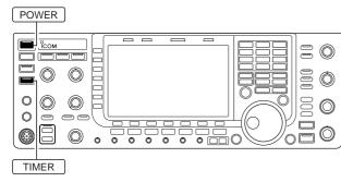
The sleep timer turns the transceiver power OFF automatically after passing the set period. The timer can be set to 5–120 min. in 5 min. steps.
