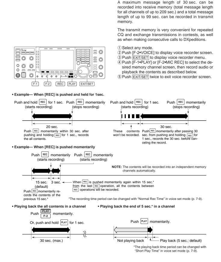
The IC-7700 has digital voice memories, up to 4 messages for transmit, and up to 20 messages for receive.
