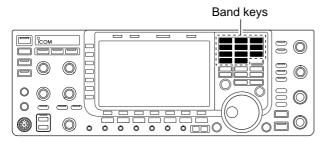
The triple band stacking register provides 3 memories for each band key, storing frequency and mode information.
