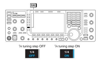
The operating frequency can be changed in larger steps (0.1, 1, 5, 9, 10, 12.5, 20 or 25 kHz selectable) for quick tuning.
