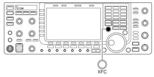
The  $\Delta$ TX function shifts the transmit frequency up to ±9.999 kHz in 1 Hz steps (10 Hz steps when cancelling the 1 Hz step readout) without moving the receive frequency.
