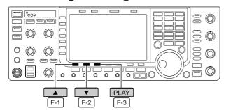
To transmit a message using the voice recorder, record the desired message in advance as described below. The IC-7700 has digital voice memories for transmission, up to 4 messages and a total message length of up to 99 sec. can be recorded.
