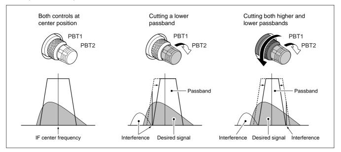
PBT (Passband Tuning) electronically narrows the IF passband width by shifting the IF frequency slightly outside of the IF filter passband to reject interference. The IC-7700 uses DSP for the PBT function. Moving both [TWIN-PBT] controls to the same position shifts the IF for both high and low frequencies.
