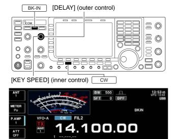
During semi break-in operation, the transceiver selects transmit when keying, then automatically returns to receive after a pre-set time after you stop sending.
