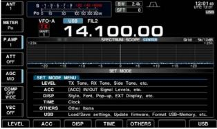
The mini scope screen can be displayed with another screen display, such as set mode menu, decode screen, memory list screen, etc. simultaneously.
