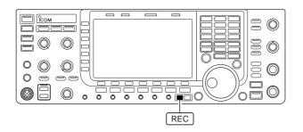
Up to 20 receive voice memories are available in the IC-7700. A total audio length of up to 209 sec. can be recorded in receive messages. However, the maximum recordable length into a single message is 30 sec.
