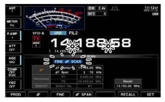
In fine scan (programmed or  $\Delta$ F), the scan speed decreases when the squelch opens, but the transceiver keeps scanning. The scanning tuning step shifts from 50 Hz to 10 Hz when the squelch opens.
