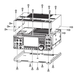
Follow the case opening procedures shown here when you want to replace the clock backup battery or internal fuse.
