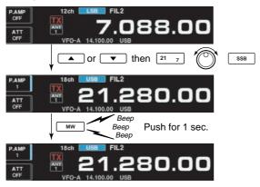
Memory channel programming can be preformed either in VFO mode or in memory mode.
