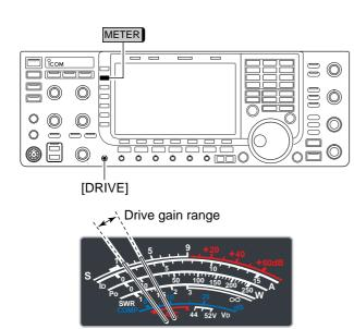
The drive gain is active for all modes other than SSB mode with speech compressor OFF. The [DRIVE] control adjusts the amplifying gain at the driver stage.
