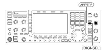
The APF changes the audio frequency response by boosting a particular frequency to enhance a desired CW signal.
