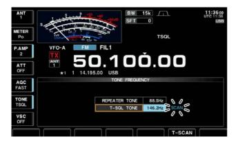
The transceiver can detect subaudible tones in a received signal. By monitoring a signal that is being transmitted on a repeater input frequency, you can determine the tone frequency required to access the repeater.
