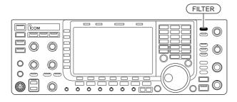
The transceiver has 3 passband width IF filters for each mode.
