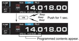
The frequency and operating mode in a memory channel can be transferred to the VFO. Frequency transferring can be performed in either VFO mode or memory mode.
