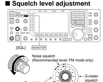
The squelch mutes noise output from the speaker (closed squelch) when no signal is received.
