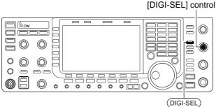
This transceiver has auto and manual notch functions. The auto notch function uses DSP to automatically attenuate more than 3 beat tones, tuning signals, etc., even if they are moving. The manual notch can be set to attenuate a frequency via the [NOTCH] control.The auto notch can be used in SSB, AM and FM mode. The manual notch can be used in SSB, CW, RTTY, PSK and AM modes.
