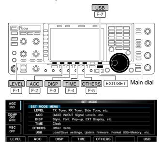
Set mode is used for programming infrequently changed values or conditions of functions. The IC-7700 has a level set mode, display set mode, time set mode, accessory set mode, Others set mode and USB-Memory set menu.
