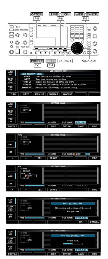
Memory channel contents, set mode settings, etc. can be saved into the USB-Memory for backup.
