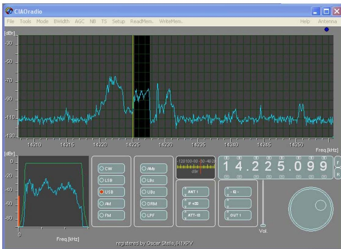
**AM** : selects amplitude demodulation . In this case the IF filter extends between  $-4\text{kHz}$  e  $+4\text{kHz}$  around the tuning frequency (yellow line). The demodulated signal is represented on a bandwidth of 8 KHz. Note: The spectrum of the demodulated signal extends outside the mask of the IF filter . The reason is because AM demodulation ( not synchronous ) is not a linear operator .
