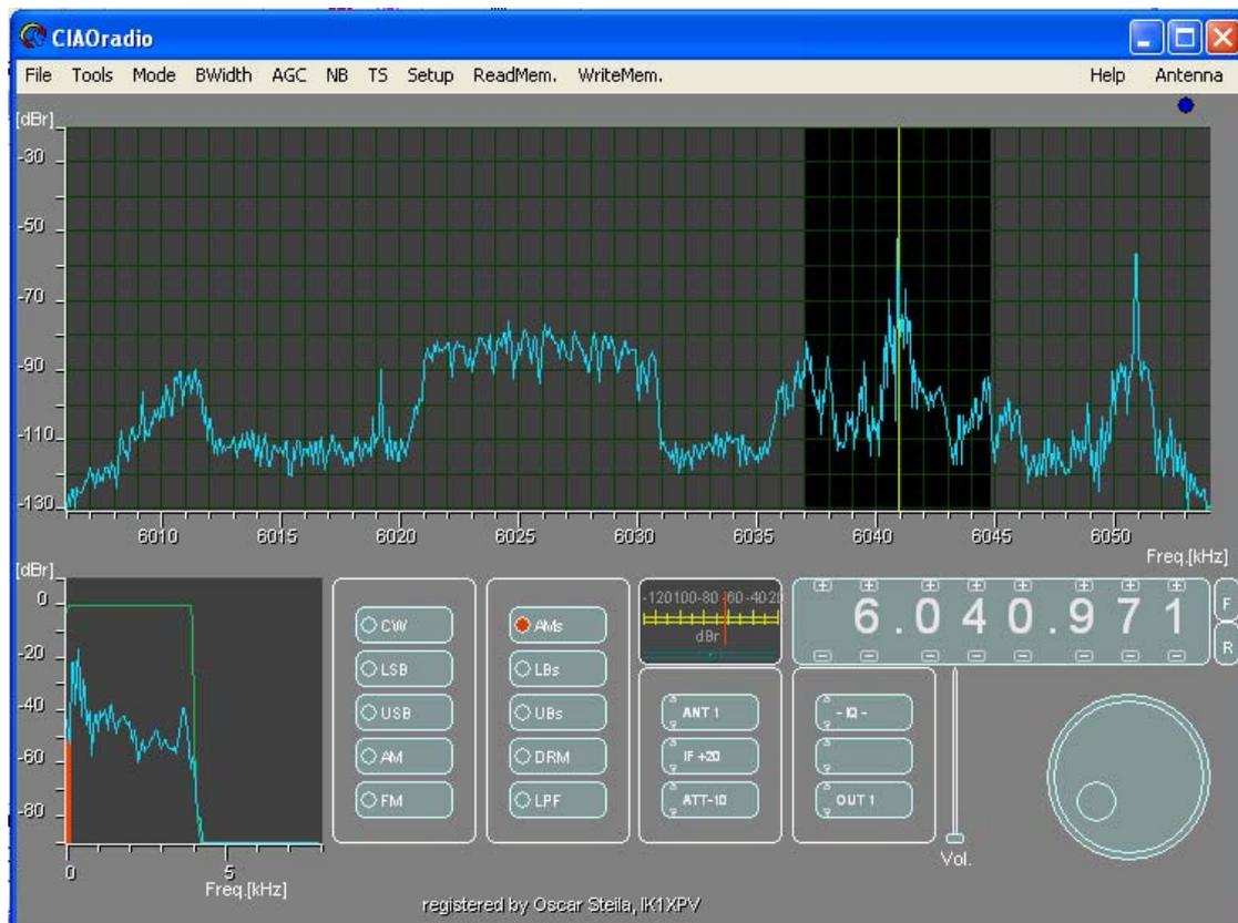
**LBs** : selects the lower side of the amplitude synchronous demodulation . In this case the IF filter extends between  $-4\text{kHz}$  e  $+25\text{Hz}$  around the tuning frequency (yellow line). The demodulated signal is represented on a bandwidth of 8 KHz. Tuning is supported from a central tuning bar on the lower part of the S-meter .
