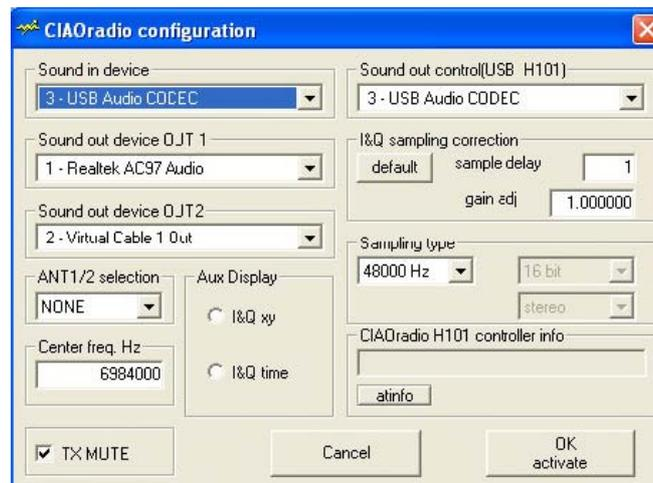
**Sound in device:** choose the input device . If H101 is installed and connected , choose the USB device, typically called “USB speakers” or “USB Audio CODEC”. It is a combobox : press the right arrow to see the sound card choice .
