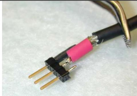
Strip approximately 1/8" from the red hookup wire and lightly tin it. Solder the tinned end to the remaining pin of the 3-pin male header plug.
