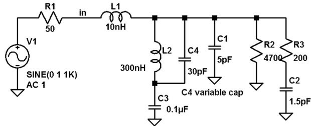
small variable plus a fixed capacitor) of about 30 pF, calculated from the normal parallel resonance formula. To avoid placing a DC short on the AD8007's input, the cold side of the parallel resonant circuit is returned to a bypass capacitor, not directly to ground.
