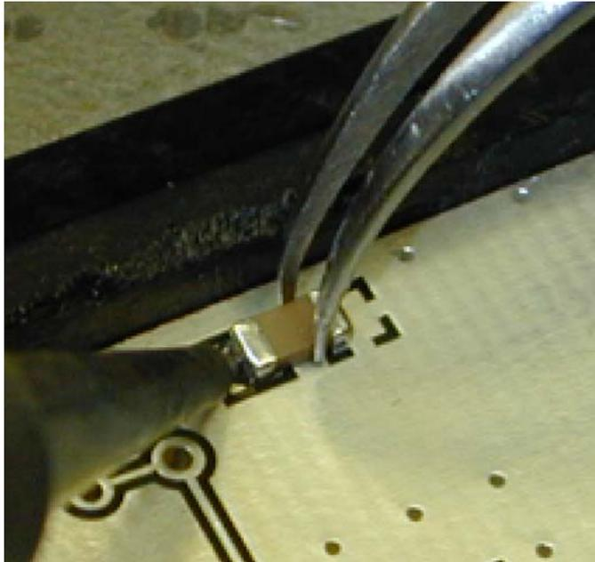
It does not take a large amount of solder to properly attach a surface mount component. A correctly installed part will be flush against the board and have a small fillet at the end caps.
