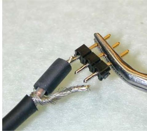
Locate the length of black heat shrink tubing in Envelope 11 and slip it over the stripped and twisted braid. Trim the tubing's length to fit.
