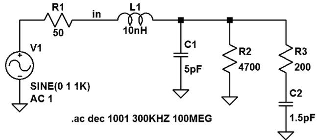
We'll start the analysis by examining a simple model of the Buffer Amplifier's input circuitry as shown at the right. This simple model does a reasonable job at modeling the Buffer Amplifier's input impedance, may be seen by comparing the computed impedance plot for the
