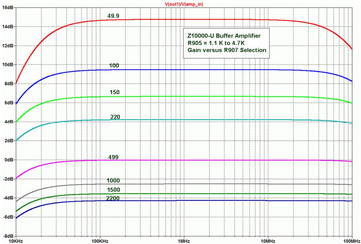
If it is necessary to operate the Z10000-U with less than -4.2 dB gain, C901 can be reduced, or in the event extreme gain reductions are required, R905 may also be reduced to provide an RC voltage divider at the amplifier's input. Although this will introduce some RC frequency shaping in the Z10000-U's frequency response, the passband tilt will be insignificant when used with a Z90 panadapter.
