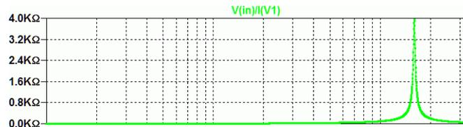
Plotting the resulting input impedance shows that at 45 MHz the input impedance is increased to about 4 KΩ. The maximum input impedance is limited by L2's Q and the R905, the 4.7 bias isolation resistor.
