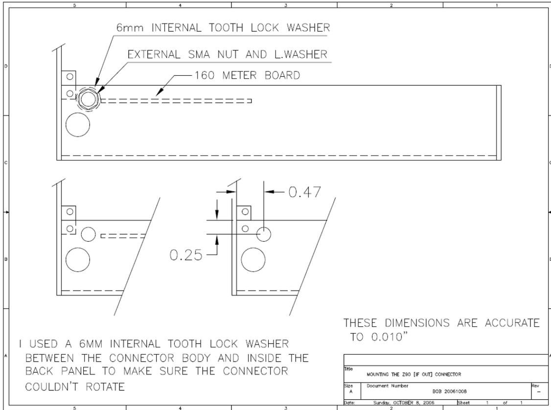
Bob notes that the 6mm (1/4") (internal diameter) lock washer just fits in between the "D" chassis bracket and the 160 Meter board so it is necessary to carefully measure the hole's location.
