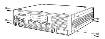
6 Attach the MB-78 to the top side of the repeater. Then tighten the 1 supplied screws (M4  $\times$  8) and 2 removed screws to each side. (6 screws at total)
