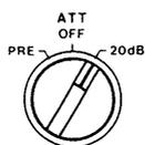
Place the [ATT] SWITCH in the [20dB] position when receiving very strong signals. In the [ATT] position, the RF preamplifier is removed from the receive path and a 20dB attenuator is inserted. This helps to reduce interference.
