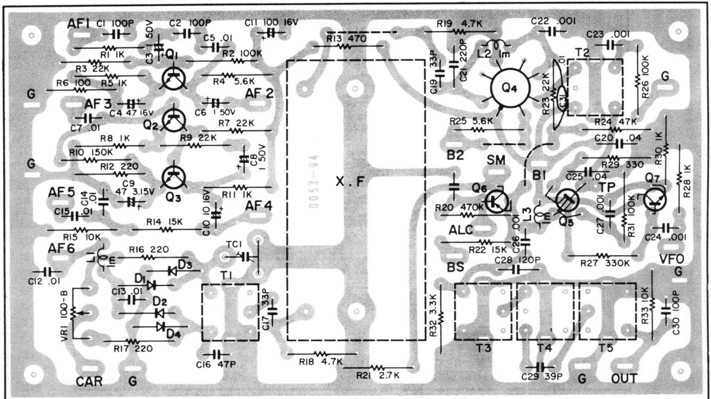
Q1: 2SC871(E), Q2,3: 2SC733(Y,GR), Q4: TA7045M, Q5: 3SK22(GR), Q6: 2SA495(Y), Q7: 2SC460(B), D1~4: 1N60
