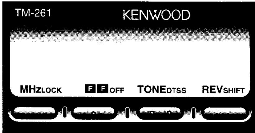
Some of the Front Panel buttons have more than one function. This allows us to provide many functions on your transceiver but keep the transceiver case small. To simplify operation, the lower portion of the Display has labels that indicate the current function of each of the 4 buttons on the lower edge of the Front Panel. The label appears immediately above its corresponding button.
