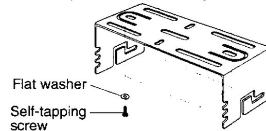
2 Position the transceiver, then insert and tighten the supplied hexagon SEMS screws and washers. There are 2 screws and 2 washers supplied for each side of the bracket.
