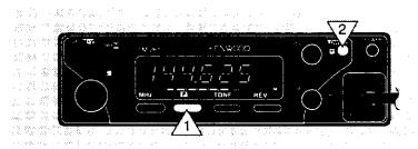
• Each time this key operation is repeated, the transmit power is changed as shown below.
