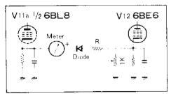
Fig5 S-Meter circuit
