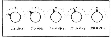
Fig19 Drive Stage Controls
