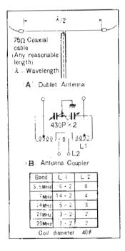
Fig12 Antenna and Antenna Coupler
