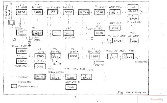
mixed with the input signal reaching Gl. They are converted by this tube to a signal whose frequency is the difference in the frequencies of the mixed signals, and range from 8.85 to 9.45 MHz. These frequencies serve as the 1st I.F. for the various bands, as shown in Table 1. A 27 PF and 10 µH series-type resonant I.F. trap which is tuned to about 9.2 MHz is provided in the Gl circuit.
