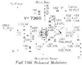
again passed through the crystal filter, and introduced to the lst transmitter Mixer. Thus, AM in actuality is A3H. The 7360 balanced modulator is quite unaffected by temperature changes. It posseses high carrier balance stability and delivers high power output. The audio characteristics curve is shown in Figure 7.
