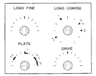
Fig15 PLATE and LOAD COARSE setting positions (with Load Impedance of 75 ohms)
