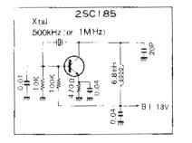
Fig16 Xtal controlled Calibrator Circuit
