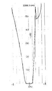
Fig4 Crystal Filter Characteristic Curve
