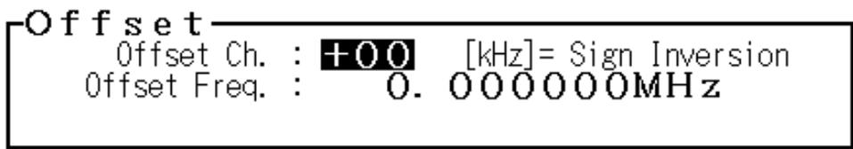
3. Rotate the **sub dial** to select the desired offset memory channel.
