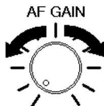
Turn clockwise to increase audio (speaker) output level and turn counterclockwise to decrease audio (speaker) output level.
