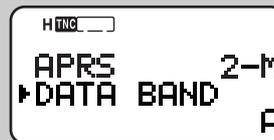
**Note:** In Menu 2-M, the selection switches among A, B, A:TX B:RX, and A:RX B:TX. Select A:TX B:RX or A:RX B:TX if APRS networks which use two separate frequencies become available in the future. "T" appears for the data transmit band and "R" appears for the data receive band.
