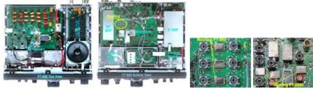
The FT-950 Front End includes new 8 Banpass Filter for radioamateur bands and no VRF (preselector) Unit;
