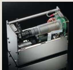
Inside the RF μ-Tune Unit
