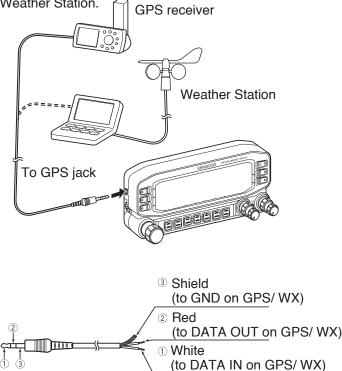
In order to use the connected GPS receiver, access Menu 602 (GPS PORT - INPUT) to select "GPS", "WEATHER ((Davis))" or "WEATHER (PeetBros.)".
