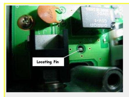
Once the rear is free, lift the board from the rear and carefully turn it upside down, towards the front. All the wiring at the front of the board is loose enough so you will not have to disconnect any of it. Here is the board being removed:
