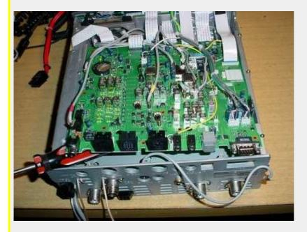
Next remove the metal shield that is below the board (10 screws):
