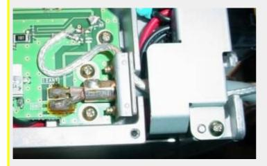
The trace is cut between the capacitor marked S1 and where the center conductor of the coax is soldered on.
