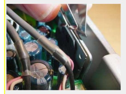
Once all 17 screws are removed, gently lift the board from the front until it is high enough to clear the locating pin at the rear of the board, shown below, and then slide the board forward until the connectors protruding through the rear panel are clear and the rear of the board can be raised.
