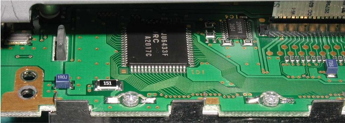
**Above:** One bank of LEDs shown with the series resistor (“151”). The anode of the diode (long lead) is on the same side as the resistor (left) for both LEDs. Make sure all 6 diodes are orientated this way! Also the LED leads must be bent back as shown. Make sure the LED sits all the way down into the hole.
