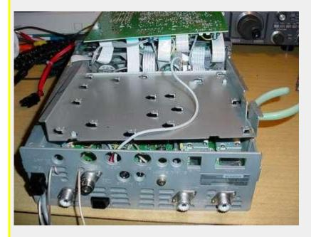
Here is the TS-2000 with the bottom board removed and ready to make the modifications:
