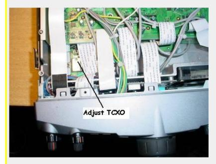
The master oscillator adjustment can be accessed from the bottom. Turn the radio upside down and remove the bottom cover. The photos show the oscillator adjustment point.
