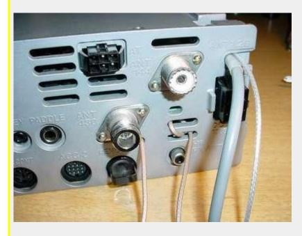
Here is a picture of the back of the modified TS-2000X, showing the three new coaxial inputs.
