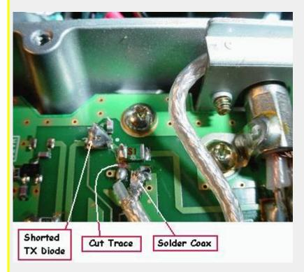
The TX diode is shorted out by a small piece of copper foil soldered across it.
