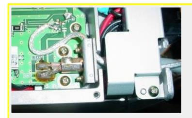
The trace is cut between the capacitor marked S1 and where the center conductor of the coax is soldered on.
