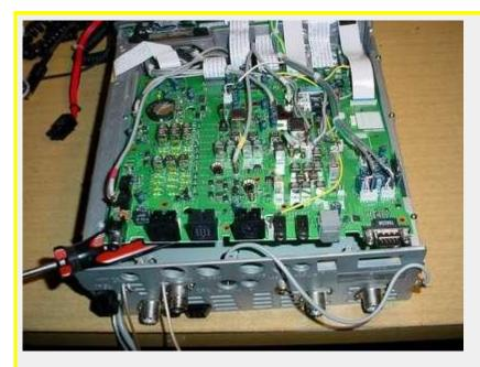
Next remove the metal shield that is below the board (10 screws):
