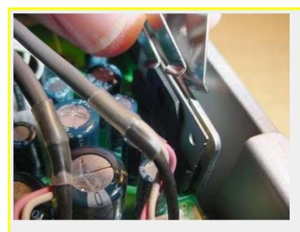
Once all 17 screws are removed, gently lift the board from the front until it is high enough to clear the locating pin at the rear of the board, shown below, and then slide the board forward until the connectors protruding through the rear panel are clear and the rear of the board can be raised.
