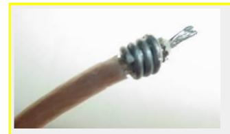
The center pin is enlarged and stiffened by soldering a short piece of solid bare wire alongside the stranded center conductor. Slightly larger solid bare wire (about #22) was wound around the shield and soldered in place to match the size of the jack that it plugs into. It only takes about a minute to make a connector like this and it works just fine.
