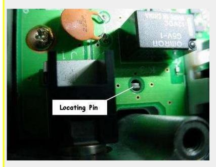
Once the rear is free, lift the board from the rear and carefully turn it upside down, towards the front. All the wiring at the front of the board is loose enough so you will not have to disconnect any of it. Here is the board being removed:
