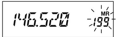
3. Within five seconds of pressing the [V/M(MW)] key, use the **DIAL** knob to select the desired memory into which you wish to store the frequency.
