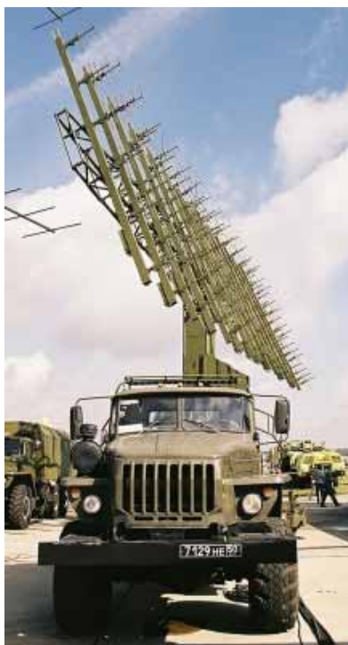
NNIIRT Nebo SVU Ural 4320 tractor towed semi-trailer variant on display in deployed configuration. Future variants are likely to employ the same BZKT 8 x 8 series chassis as the newer Nebo M component radars (Images © Miroslav Gyúrosi ).
