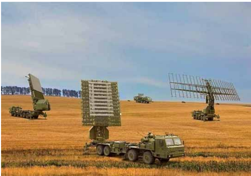
Rendering of Almaz-Antey/NNIIRT 55Zh6ME Nebo ME deployed. The VHF-band component is at the right of the image, the S/C-band component is at the left of the image, the
