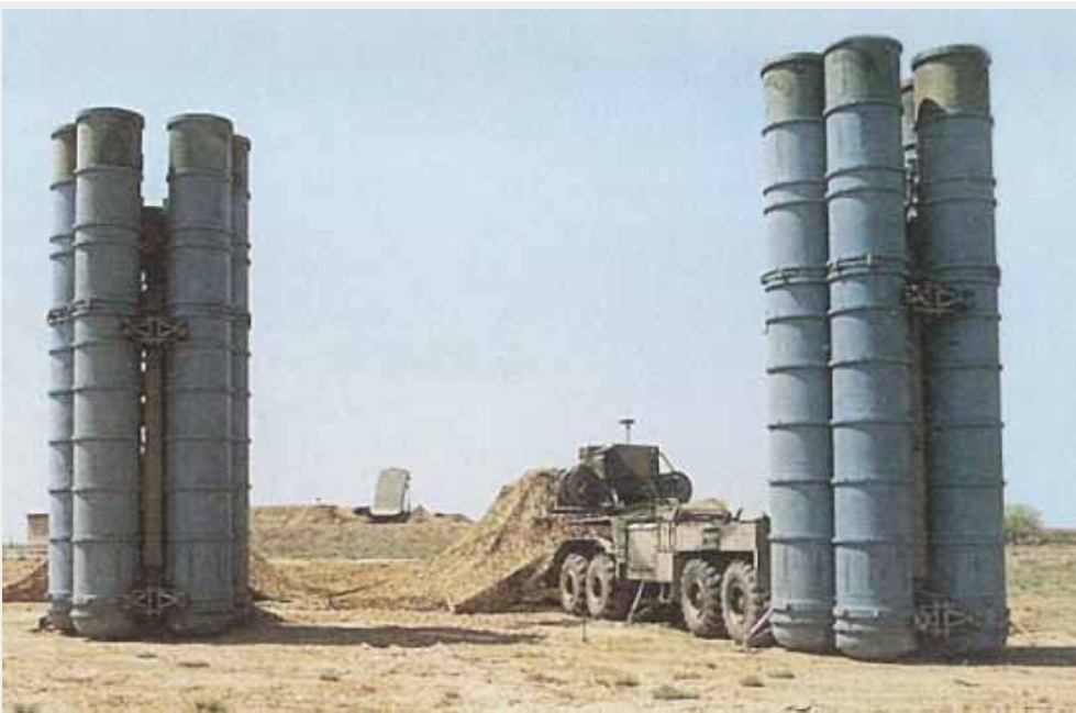
Deployed S-300PMU2 Favorit / SA-20B Gargoyle battery. The 30N6E2 Flap Lid engagement radar is visible in the distance . This battery is networked via cables, and the telescoping network antennas are retracted (RuMOD).
