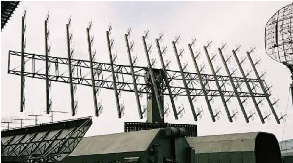
Above, NNIIRT 1L119 Nebo SVU on display at MAKS2003. These images are very revealing insofar as they clearly show the combination of 3/8 folded dipoles and directors in a regular grid array. Below, detail of outermost left pair of array element columns, showing 3/8 dipole and director in detail (Images © Miroslav Gyűrösi).
