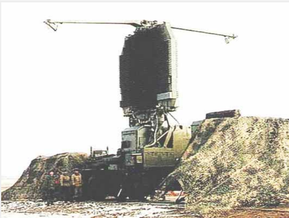
NIIP 64N6E Big Bird deployed. This Aegis-like 2 GHz band dual faced transmissive PESA acquisition radar is the core of late model S-300PMU2 Favorit / SA-20 Gargoyle and in its 91N6E variant, the S-400 Triumph / SA-21 missile battery. The radar can be deployed/stowed for "shoot and scoot" operations in a mere 5 minutes. Stated tracking accuracy is 200 metres in range, 30 min in azimuth, and 35 minutes in elevation.
