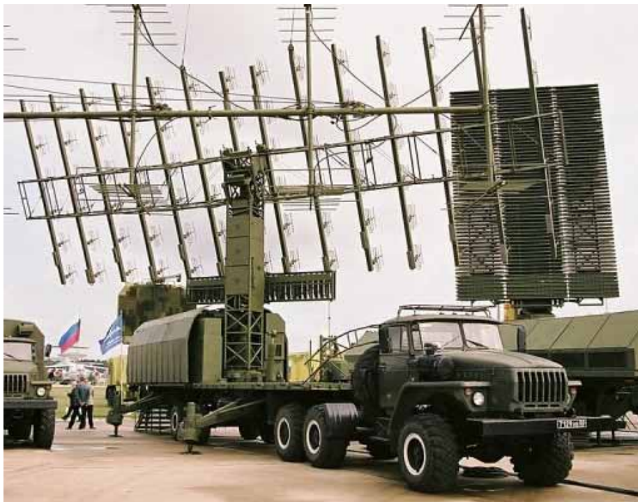
NNIIRT Nebo SVU Ural 4320 tractor towed semi-trailer variant on display in deployed configuration. Future variants are likely to employ the same BZKT 8 x 8 series chassis as the newer Nebo M component radars (Images © Miroslav Gyúrosi ).
