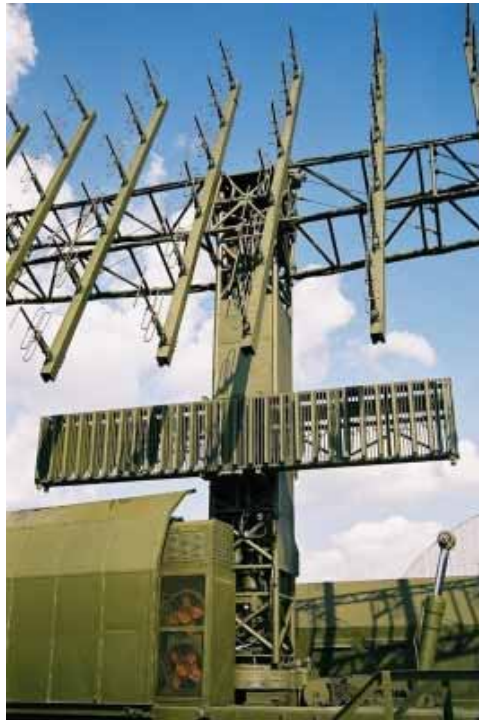
Detail of antenna mast, IFF array, and primary antenna. Note the tilt actuator and joint, and the turntable at the base of the mast (Images © Miroslav Gyűrösi).
