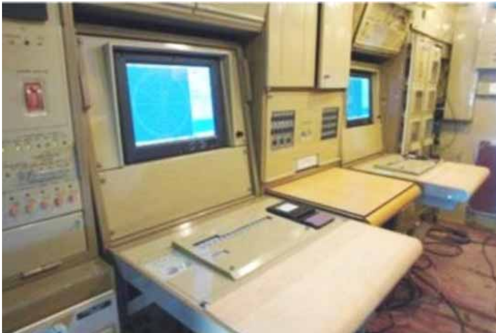
The 1L119 Nebo SVU makes full use of modern COTS technology, with 17 inch LCD displays for operators (above), and flexible digital display presentation (below). Display formats can include geographical data such as borders, air defence zones, and range boundaries (NNIIRT).
