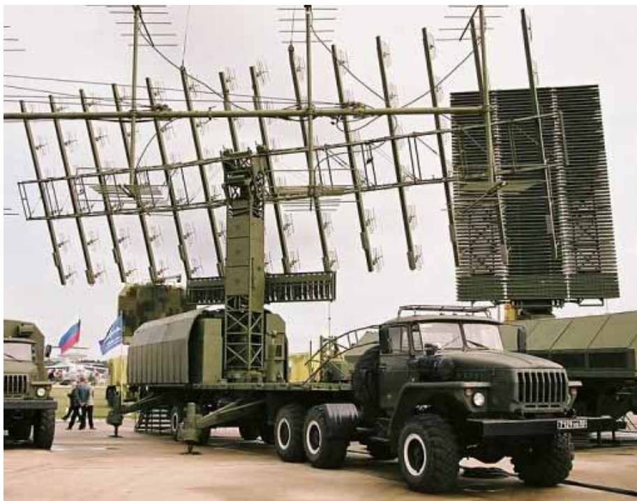
NNIIRT Nebo SVU Ural 4320 tractor towed semi-trailer variant on display in deployed configuration. Future variants are likely to employ the same BZKT 8 x 8 series chassis as the newer Nebo M component radars (Images © Miroslav Gyürösi ).
