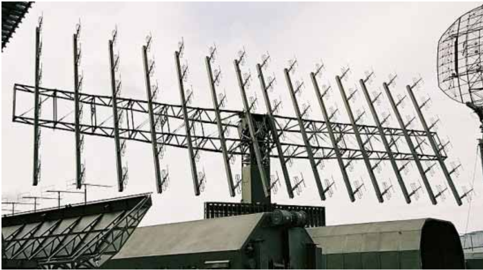
Above, NNIIRT 1L119 Nebo SVU on display at MAKS2003. These images are very revealing insofar as they clearly show the combination of 3/8 folded dipoles and directors in a regular grid array. Below, detail of outermost left pair of array element columns, showing 3/8 dipole and director in detail (Images © Miroslav Gyürösi ).
