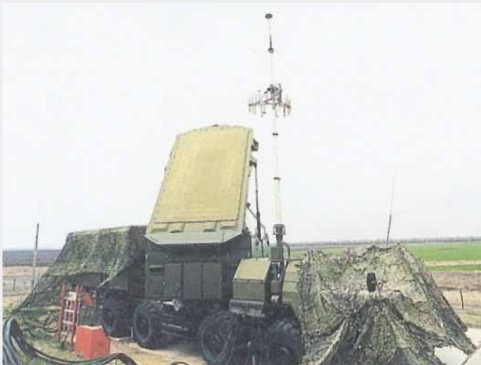
S-300PMU 30N6E Tomb Stone engagement radar in deployed configuration. This X-band system provides midcourse guidance and Track Via Missile terminal homing for the Fakel 48N6E missiles, and in later variants midcourse guidance for the active radar seeker equipped Fakel 9M96E/E2 missiles. There are no fundamental technological obstacles to integration with the 1L119 Nebo SVU, using the latter as a source for a midcourse update target coordinate data feed. Note the telescoping omni-directional network antenna (RuMOD).
