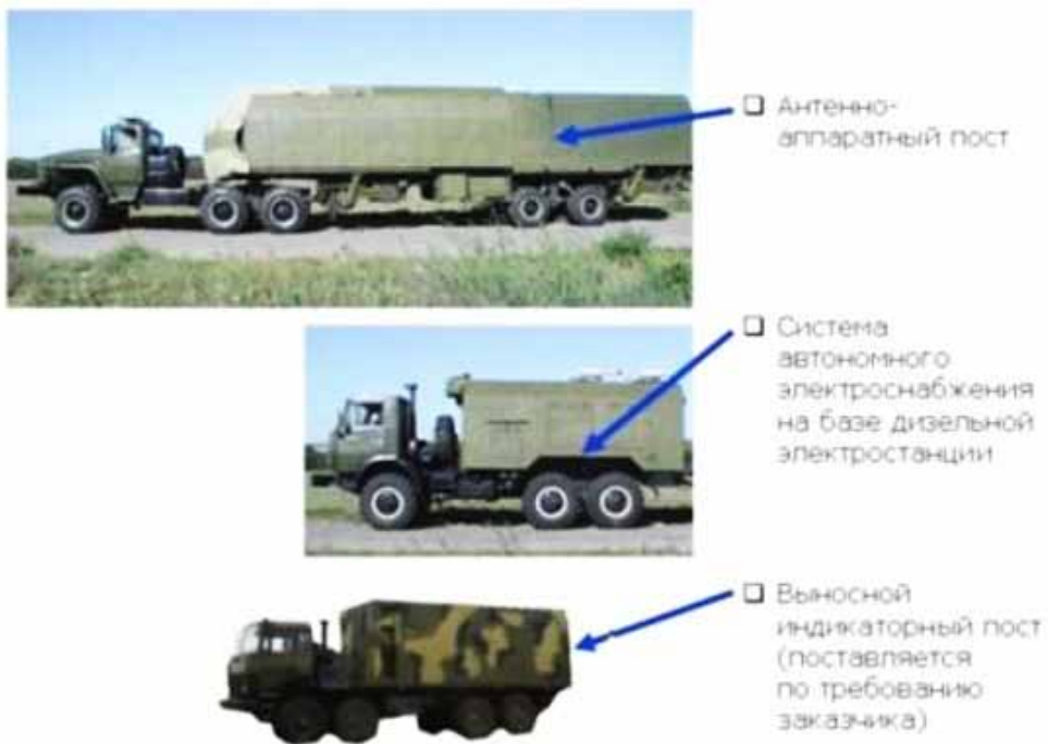
Stowed configuration. The Nebo SVU occupies three vehicles. A semitrailer carries the antenna/radar system, a 6x6 truck the diesel generators, and a 4x4 truck the operator cabin. The system can be deployed in 20 minutes, which is less than half of the time required for other Russian VHF radars (NNIIRT).
