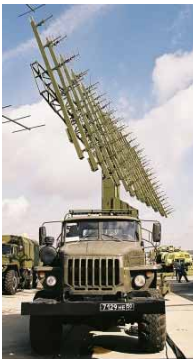
NNIIRT Nebo SVU Ural 4320 tractor towed semi-trailer variant on display in deployed configuration. Future variants are likely to employ the same BZKT 8 x 8 series chassis as the newer Nebo M component radars (Images © Miroslav Gyürösi ).
