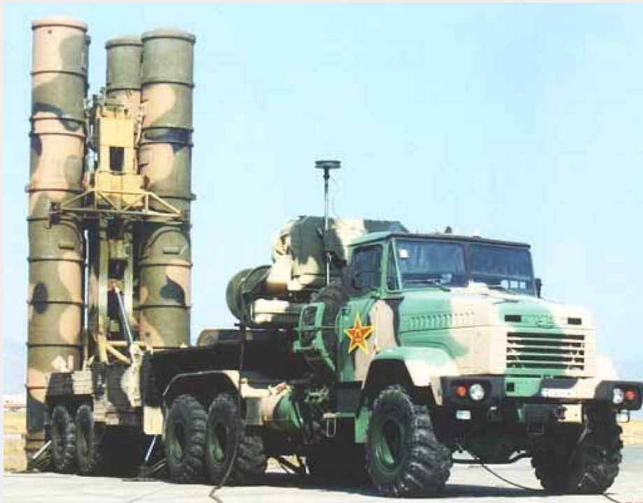
S-300PMU-2 Favorit / SA-20 Gargoyle 5P85TE TEL in deployed configuration, with the telescoping network antenna retracted. The PLA remains the largest export customer for S-300PMU variants (Xinhua).
