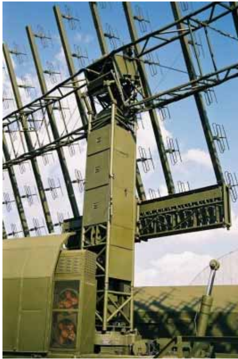
Detail of antenna mast, IFF array, and primary antenna. Note the tilt actuator and joint, and the turntable at the base of the mast (Images © Miroslav Gyűrösi).
